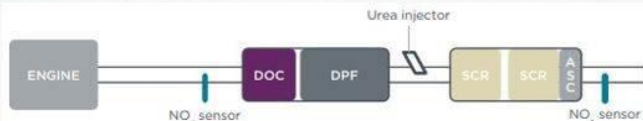
Figure 1. EPA 2010 aftertreatment system layout.
