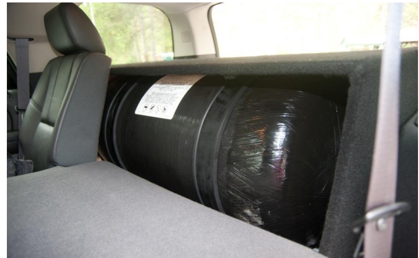
CNG tank located in the back of a Tahoe
