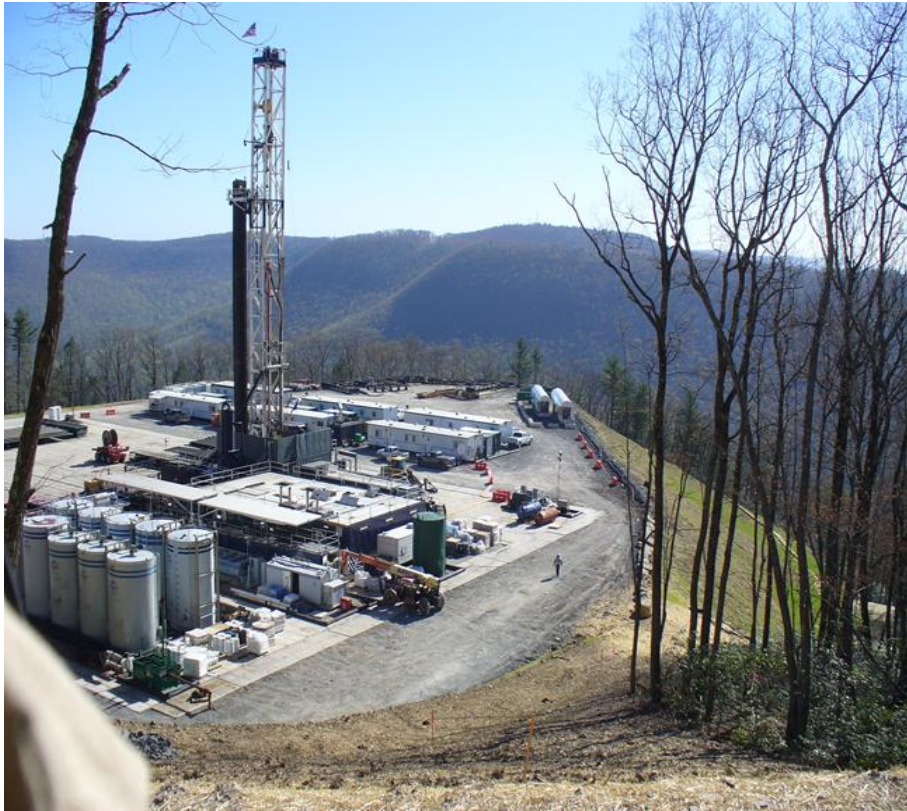
Ensign Rig # 125 at DCNR 100, Pad T, Lycoming County, PA Prometheus LNG vaporizer & storage tanks are in upper right
